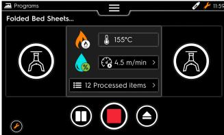
You can use the machine and see the diiferent status of the feeder clamps or the heating and speed.
