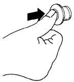
Release the emergency stop, by turning it clockwise only after checking what motivated this stop.
